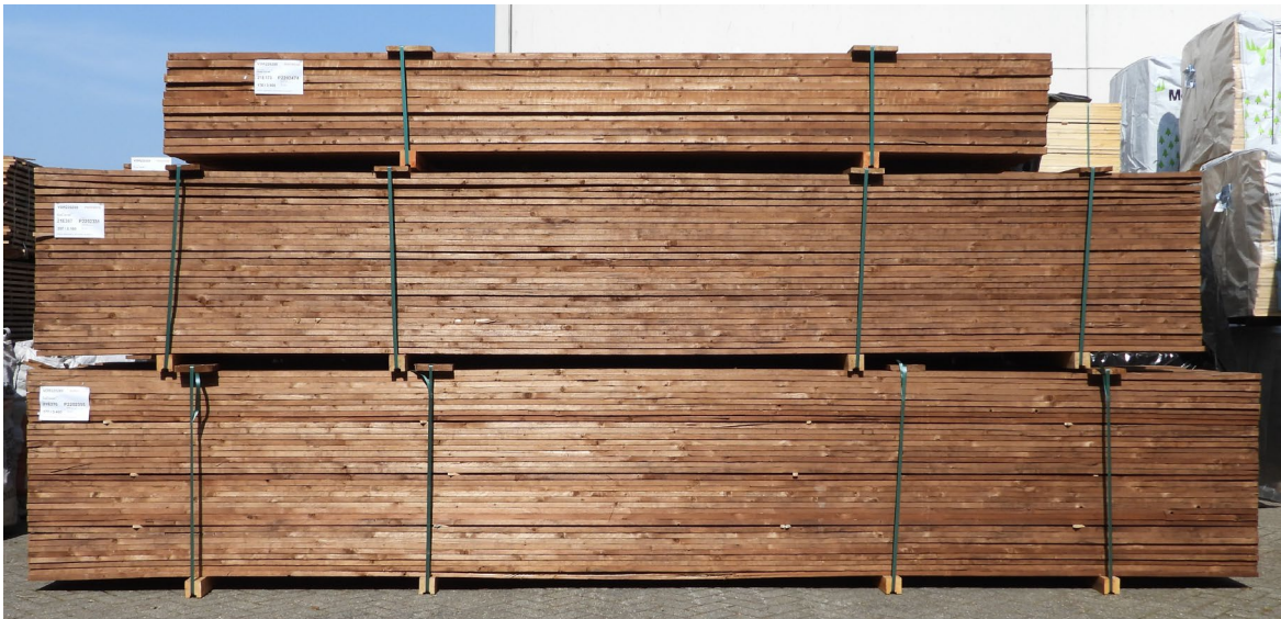
Figure 1 – Store untreated wood in the correct way
